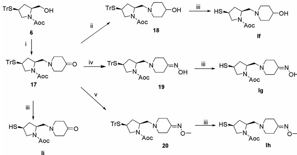
**Reactions and conditions:** (i) 1.) Trifluoromethane sulfonic anhydride, CH<sub>2</sub>Cl<sub>2</sub>, 2.) 16, TEA, CH<sub>2</sub>Cl<sub>2</sub>; (ii) NaBH<sub>4</sub>, THF; (iii) Trifluoroacetic acid, triethylsilan, CH<sub>2</sub>Cl<sub>2</sub>; (iv) Hydroxylamine, EtOH; (v) Methoxyamine hydrochloride, pyridine.
