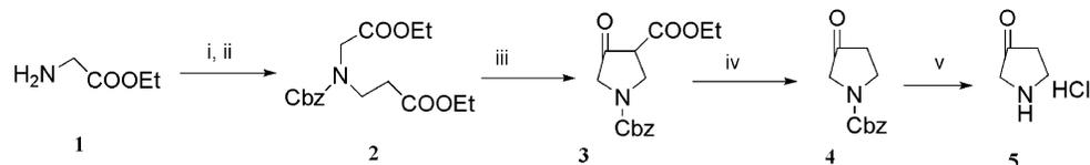
**Reactions and conditions:** (i) Ethyl acrylate, TEA, EtOH; (ii) Benzyl chloroformate, TEA, CH<sub>2</sub>Cl<sub>2</sub>; (iii) Potassium *t*-butoxide, toluene; (iv) 10% HCl; (v) Pd/C, H<sub>2</sub>, EtOH.
