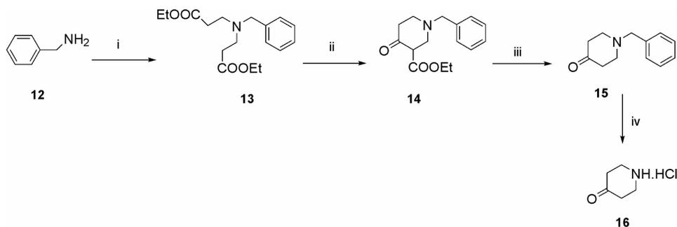
**Reactions and conditions:** (i) Ethyl acrylate, TEA, EtOH; (ii) NaH, toluene; (iii) 10% HCl; (iv) Pd/C, H<sub>2</sub>, EtOH.
