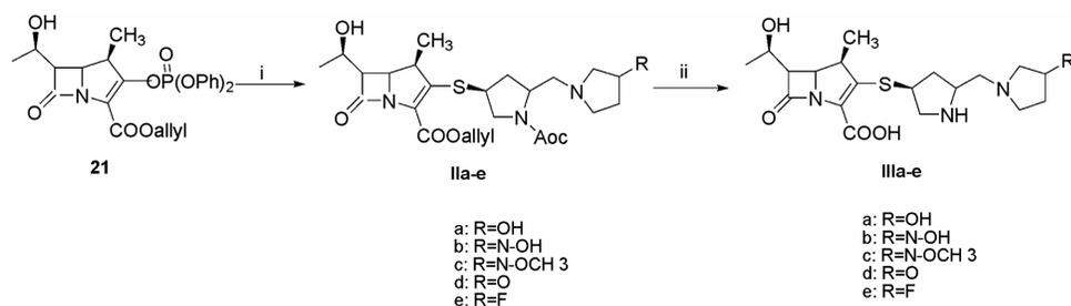
**Reactions and conditions:** (i) *N,N*-Diisopropylethyl amine, Ia–e; (ii) Tetrakis(triphenylphosphine)palladium, tributyltin hydride, CH<sub>2</sub>Cl<sub>2</sub>.
