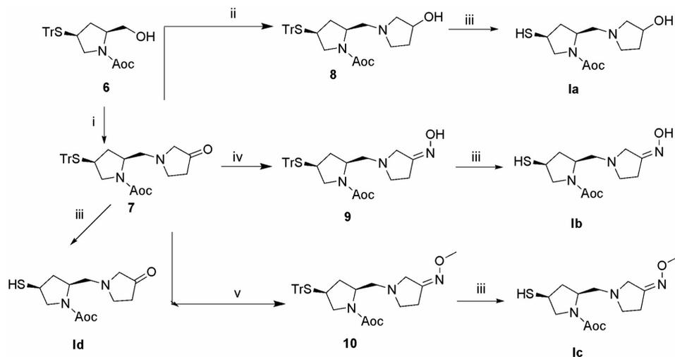
**Reactions and conditions:** (i) 1.) Trifluoromethane sulfonic anhydride, CH<sub>2</sub>Cl<sub>2</sub>, 2.) **5**, TEA, CH<sub>2</sub>Cl<sub>2</sub>; (ii) NaBH<sub>4</sub>, THF; (iii) Trifluoroacetic acid, triethylsilane, CH<sub>2</sub>Cl<sub>2</sub>; (iv) Hydroxylamine, EtOH; (v) Methoxyamine hydrochloride, pyridine.
