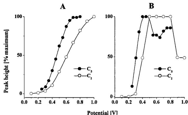
**Figure 4.** Voltage dependence of HPLC-EC signals of PBN/ $C_2H_5$  and PBN/ $C_5H_{11}$ . Both hydroxylamine (A) and nitroxide (B) forms of the adducts were subjected to EC-HPLC analysis at different holding potential. The nitroxide and their hydroxylamine derivatives were prepared as described in the Materials and Methods and diluted 10 times in ethanol prior to HPLC separation.
