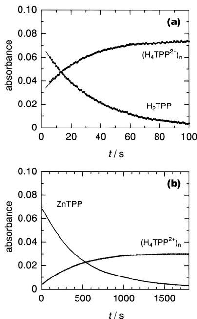
Figure 3. First-order kinetic profiles observed from the CLM measurements in the diprotonation of  $H_2TPP$  (a) and the demetalation of  $ZnTPP$  (b). The solid line is the fitting curve obtained by the first-order analysis. The initial concentrations of  $H_2TPP$  and  $ZnTPP$  were  $1.71 \times 10^{-5}$  and  $8.9 \times 10^{-6} \text{ mol dm}^{-3}$ , respectively. The concentration of hydrochloric acid was  $2.0 \text{ mol dm}^{-3}$ .
