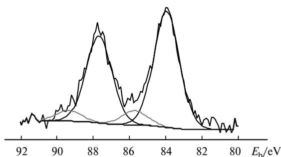
Fig. 3. Deconvolution of the photoelectron Au4f spectrum of the Au(3.5%)/Ch—SiO<sub>2</sub> sample.
