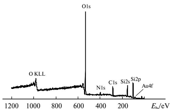
Fig. 1. XPS review spectrum of the Au(3.5%)/Ch—SiO<sub>2</sub> sample;  $E_b$  is the binding energy.
