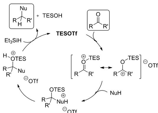
Scheme 5. Proposed simplified catalytic cycle based on TESOTf as active catalyst.
