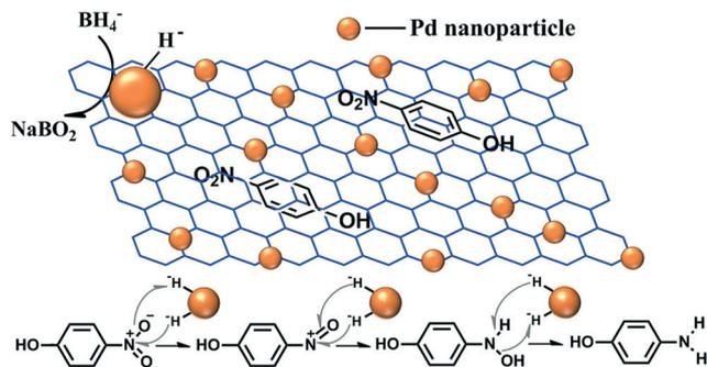
**Scheme 1** A plausible mechanism for the reduction of *p*-nitrophenol catalyzed by the Pd/G catalyst in the presence of sodium borohydride.
