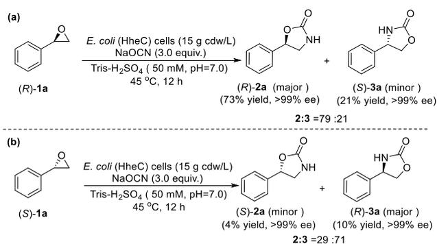
**Scheme 2.** Investigation of bioconversions of (*R*)-**1a** and (*S*)-**1a** catalyzed by HheC. Reaction conditions: Tris-H<sub>2</sub>SO<sub>4</sub> buffer (pH 7.0, 50 mM, 30 mL), *E. coli* (HheC) cells (15 g cdw/L), (*R*)-**1a** or (*S*)-**1a** (30 mM), NaOCN (90 mM), 45 °C and 12 h. The yields of **2a** were isolated by column chromatography; the yields of **3a** were calculated from the yield of **2a** by <sup>1</sup>H NMR.
