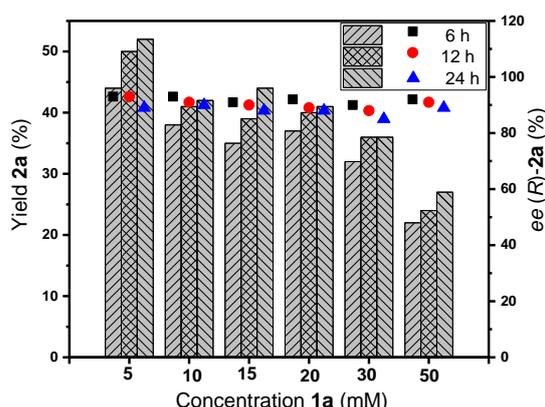
**Figure 1.** Investigation of substrate concentrations. Reaction conditions: Tris-H<sub>2</sub>SO<sub>4</sub> buffer (50 mM, pH 7.0, 5 mL); *E. coli* (HheC) cells (15 g cdw/L), **1a** (5–50 mM), NaOCN (15–150 mM), 45 °C. The yield (column) and ee (scatter) were determined over the formed product at 6, 12 and 24 h by chiral HPLC.
