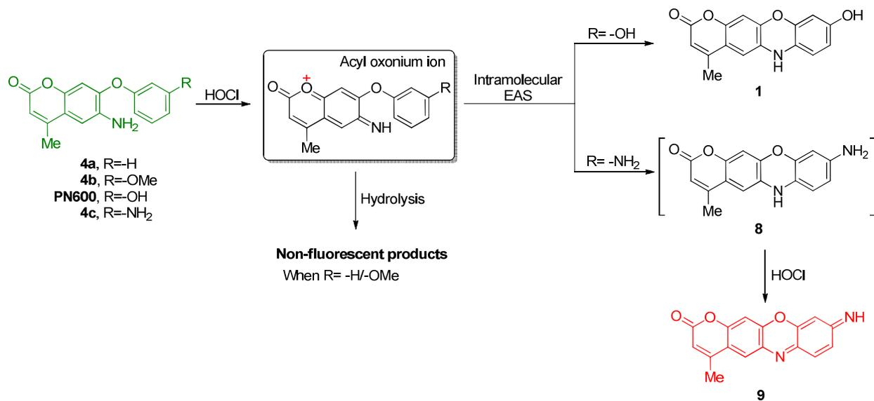
Figure 6: Proposed oxidation schemes for **4a**, **4b**, **PN600** and **4c** by hypochlorite, based on titrations shown in Figure 5.
