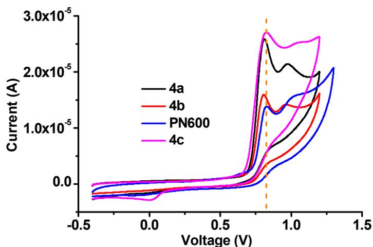
Figure 7. Cyclic voltammograms of probes **4a**, **4b**, **PN600** and **4c** in DMF.
