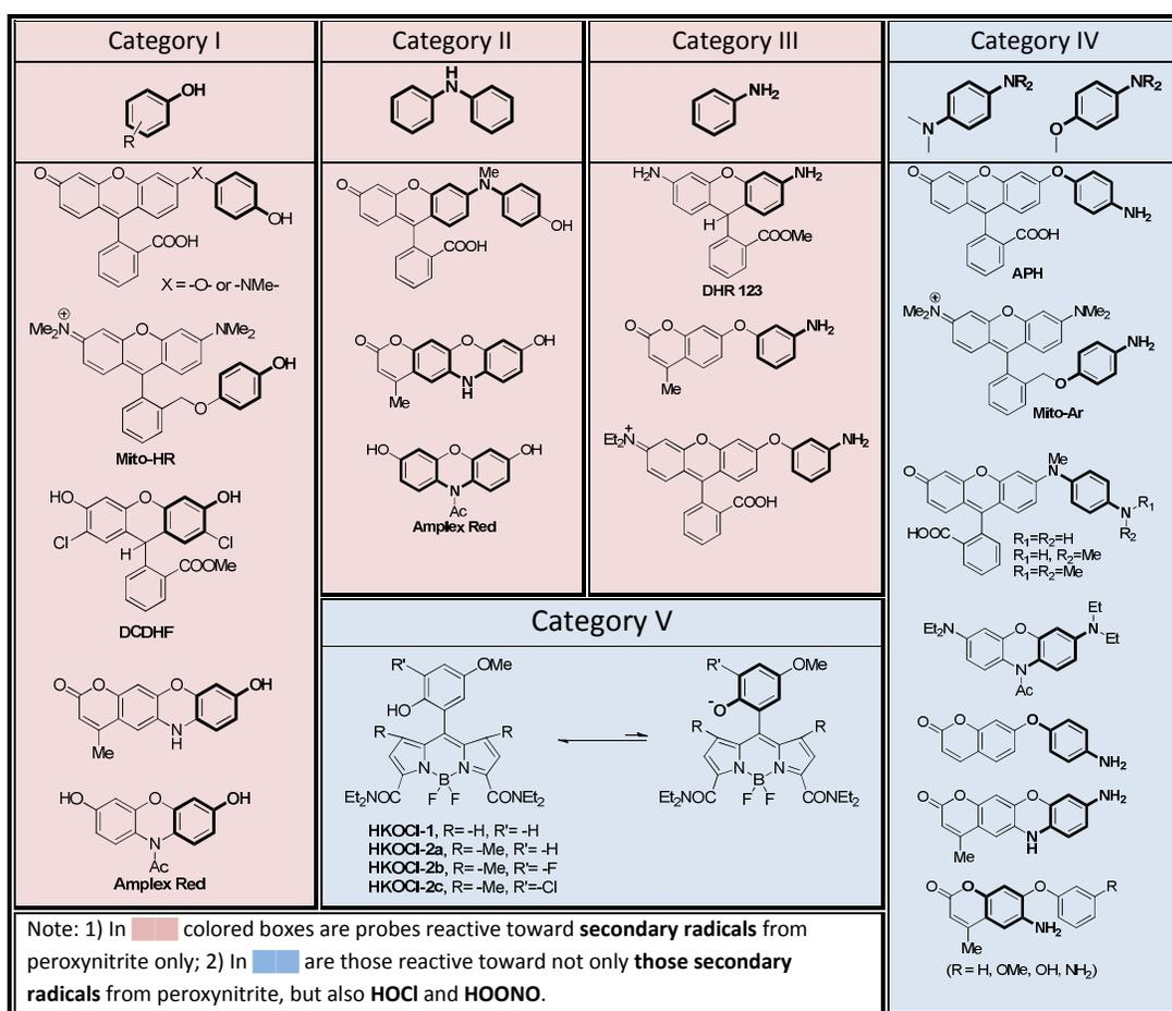
**Chart 1: Classification of probes for hypochlorite and peroxynitrite based on oxidation of an electron-rich aromatic ring.**
