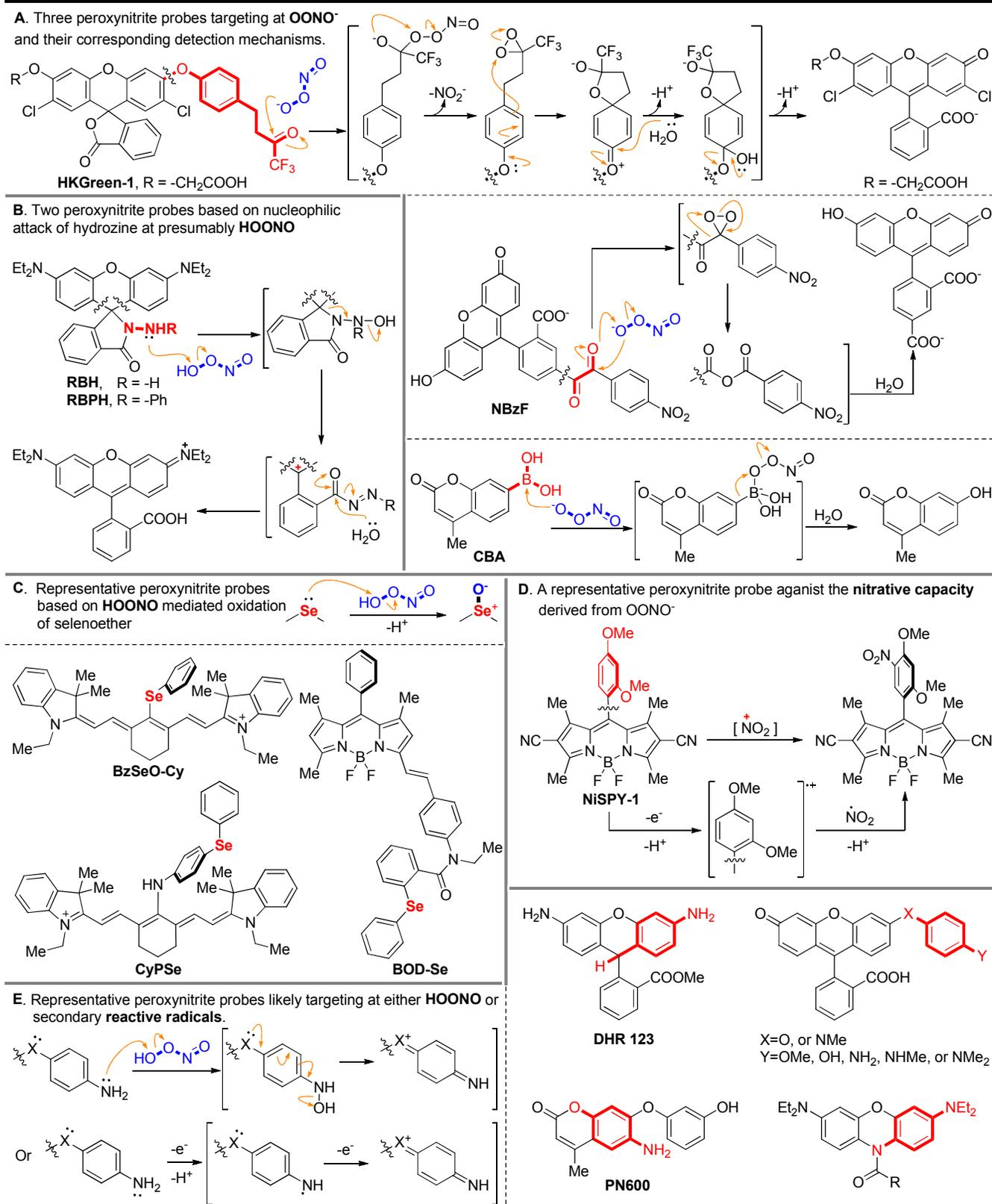
Figure 2: Classification of existing peroxyxynitrite probes by their detection mechanisms.
