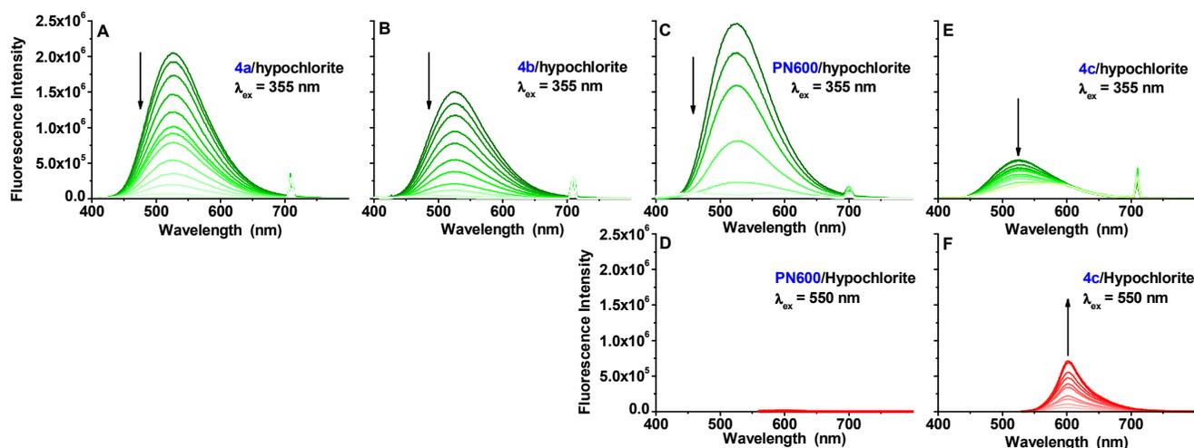
Figure 5: Fluorescence titrations of probes **4a**, **4b**, **PN600** and **4c** by hypochlorite. Excitation was set at 355 nm to monitor the decrease of the probe emission of **4a** (A), **4b** (B), **PN600** (C) and **4c** (E) upon addition of hypochlorite. Excitation was set at 550 nm to monitor the formation of **2** from **PN600** (D), and **9** from **4c** (F) upon addition of hypochlorite.
