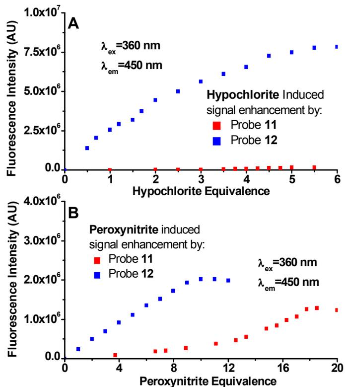
Figure 13. Dose dependent fluorescence enhancement of probes **11** and **12** by hypochlorite (A) and peroxyntirite (B).
