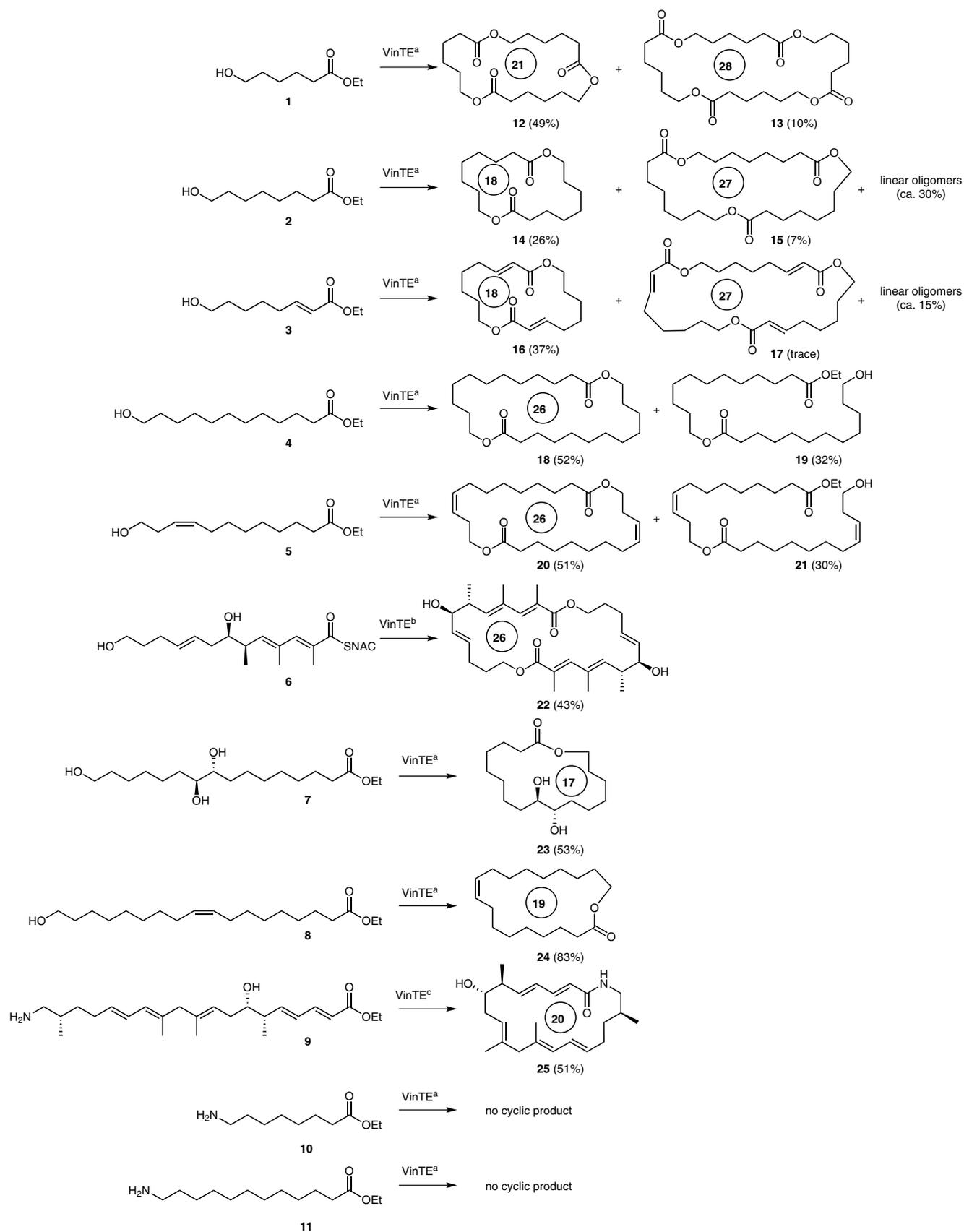
**Scheme 2** VinTE reaction with  $\omega$ -hydroxy fatty acid ethyl esters. <sup>a</sup> 60  $\mu\text{M}$  of VinTE, 1–3 mM of substrate, 28  $^\circ\text{C}$ , 24 h; <sup>b</sup> 300  $\mu\text{M}$  of VinTE, 7 mM of substrate, 28  $^\circ\text{C}$ , 24 h. <sup>c</sup> 130  $\mu\text{M}$  of VinTE, 1.25 mM of substrate, 28  $^\circ\text{C}$ , 40 min.<sup>6</sup>
