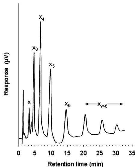
Fig. 3. Pattern of xylo-oligosaccharides released from soluble xylan by endo- $\beta$ -1,4-xylanase from *S. thermophile* ATCC 34628.
