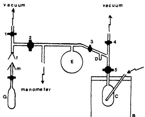
Figure 3. Apparatus for pyrolysis of cyclopropane: (A) thermocouple well; (B) molten salt bath; (C) reaction chamber; (D) freeze-out bulb; (E) 200 ml reservoir; (G) sample storage vessel; (1–4) glass stopcocks; (5) high-vacuum Teflon stopcock; (f and m) female and male standard taper joints.
