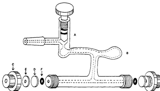
**Figure 4.** Pressure cell for polarimetry: (A) Teflon high-vacuum stopcock; (B) reservoir; (C) screw cap; (D) silica window; (E) Teflon spacer; (F) Buna N rubber O ring.
