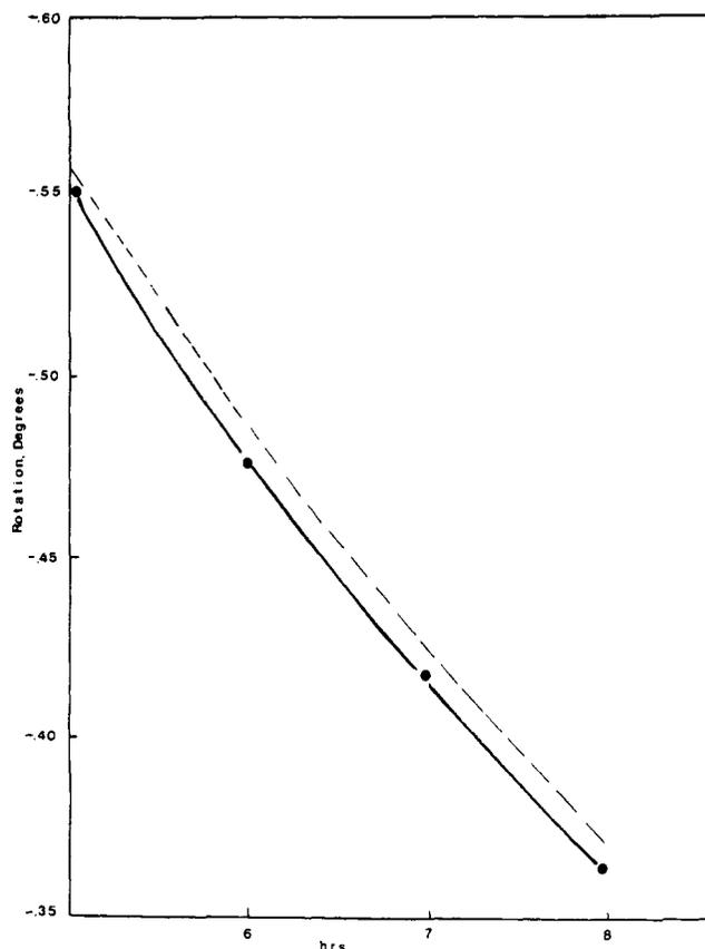
Figure 2. Loss of optical activity in the pyrolysis of (-)-*trans*-1-phenylcyclopropane-2-*d*. Only the later experimental kinetic points are shown (circles). Both curves are calculated using  $k_H/k_D = 1.10$ . The dashed curve is for  $k_1 = 0.395 \times 10^{-5} \text{ sec}^{-1}$ ; the solid one is for  $k_1 = 0$ .
