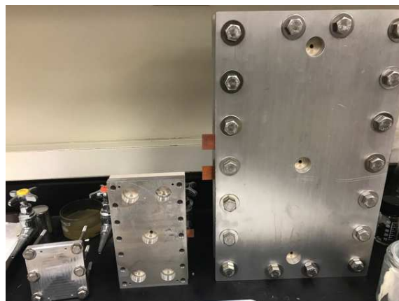
Figure 2. Three sizes of flow electrolysis cells.
