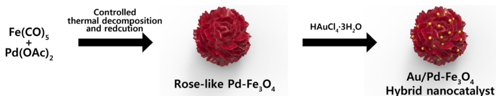
Scheme 5. Synthetic scheme of Au/Pd-Fe 3 O 4 nanocomposites.
