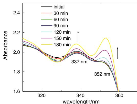
**Fig. 4.** In situ UV-vis spectra of Ru(bppb)(pydic) in the oxidation of diphenylmethane with TBHP.
