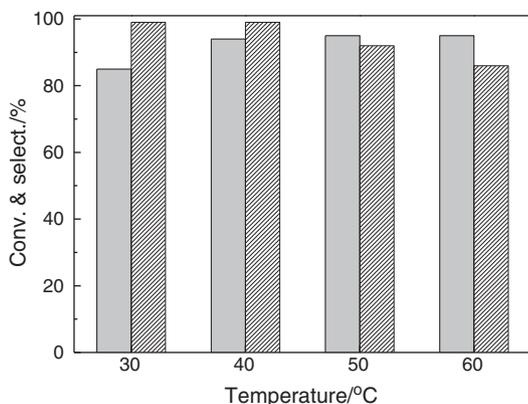
**Fig. 1.** Effect of temperature on the conversion of diphenylmethane (■), selectivity of benzophenone (▨), reaction conditions: diphenylmethane (1 mmol), catalyst ( $1 \times 10^{-4}$  mmol), ethyl acetate (3 mL), TBHP (3 mmol), 5 h.
