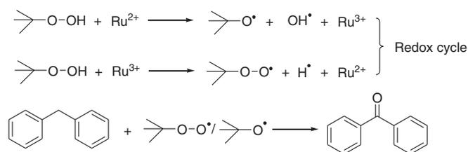
**Scheme 2.** The proposed mechanism for the oxidation of diphenylmethane catalyzed by Ru(bppb)(pydic).
