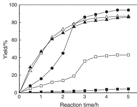
**Fig. 3.** The oxidation of diphenylmethane with different catalyst/substrate molar ratios over Ru(bppb)(pydic). (■): 0, (□): 1/100,000, (●): 1/10,000, (▲): 1/1,000, (△): 1/100, reaction conditions: diphenylmethane (1 mmol), ethyl acetate (3 mL), TBHP (3 mmol).
