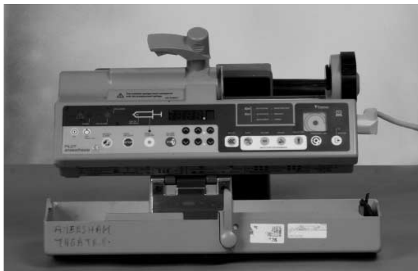
Figure 6 Behind the façade of the 'Diprifusor' pump is a syringe driver.
