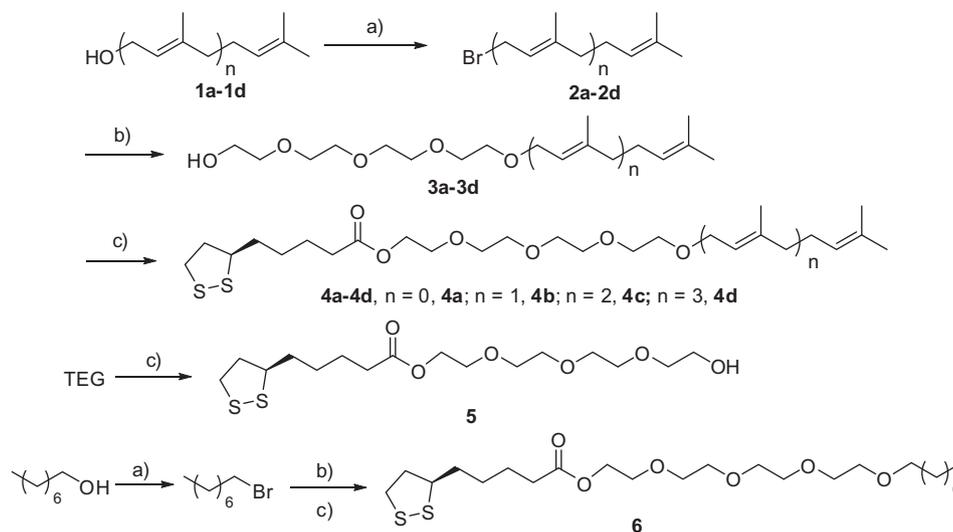
**Scheme 1.** Synthesis of probes. Reagents and conditions: (a)  $\text{CBr}_4$ ,  $\text{PPh}_3$ ,  $\text{DCM}$ , 60–89%; (b) TEG, NaH, DMF, 0 °C, 45–71%; (c) DMAP/EDC, liponic acid, DMF, 30 °C, 35–92%.
