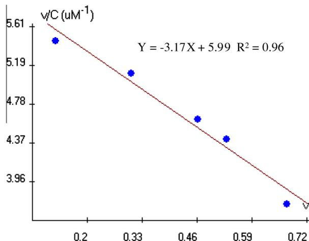
**Figure 2.** Scatchard plot of 3PGK affinity binding to **4b**. The quartz chip was modified by a **4b** and **5** mixture in a molar ratio of 2:1. V:  $\Delta F/\Delta F_{\text{max}}$ , C: concentration of 3PGK.
