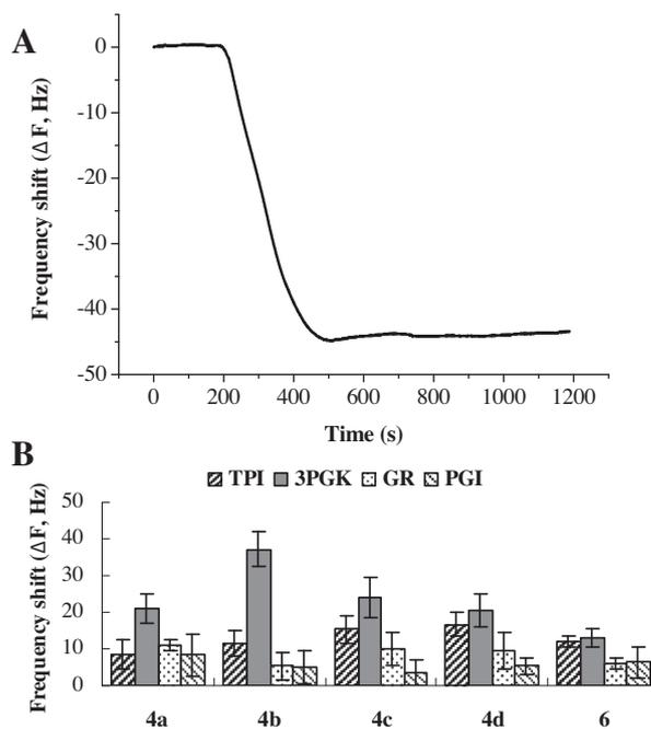
**Figure 1.** QCM analysis molecular interactions between synthetic probes and proteins. (A) The saturation binding curve over time of 3PGK interacting with **4b**. (B) Frequency shifts of interaction of probes **4a-d** and **6** with proteins. All quartz chips were modified by a mixture of indicated probe and **5** (mol/mol, 2:1). Concentrations of 3PGK, TPI, GR, and PGI were 200, 100, 54, and 120  $\mu\text{g/ml}$ , respectively.
