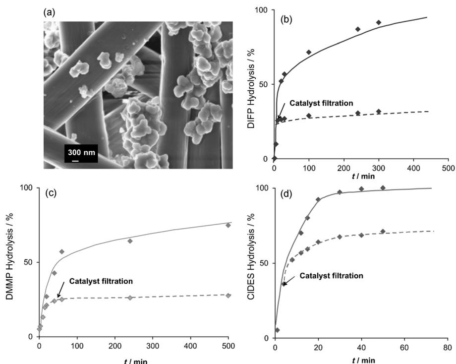
**Figure 6.** a) VP-SEM (VP=variable pressure) images of silk@[UiO-66@LiOtBu] composite. Hydrolytic degradation profiles of b) DIFP, c) DMMP, and d) CEES, all catalyzed by silk@[UiO-66@LiOtBu] composite at room temperature. The dotted lines indicate the effect of removing the [UiO-66@LiOtBu] by filtration to demonstrate the heterogeneity of the catalytic process.
