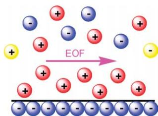
Figure 2. Schematic illustrating the principle of electroosmotic flow.
