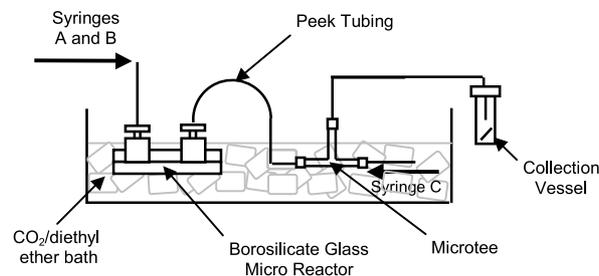
Figure 16. Schematic of the reaction set-up used for the evaluation of reduced temperature micro reactions.
