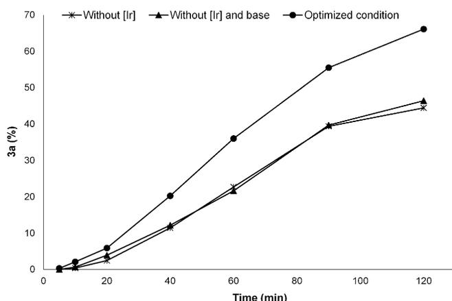
**Figure 2.** Reaction profile that shows the amount of amide **3a** formed. Reaction conditions: **1a** (0.25 mmol, 1.0 equiv.), **2a** (2.0 equiv.), 115°C. The progress in the reaction was monitored by GC analysis using dodecane as the internal standard.
