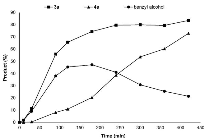
**Figure 1.** Reaction profile that shows the amount of product formed. Reaction conditions: **1a** (0.25 mmol, 1.0 equiv.), **2a** (2.2 equiv.),  $[\text{Cp}^*\text{IrCl}_2]_2$  (1.25 mol%), NaOAc (2.5 mol%), 115 °C. The progress in the reaction was monitored by GC analysis using dodecane as the internal standard.
