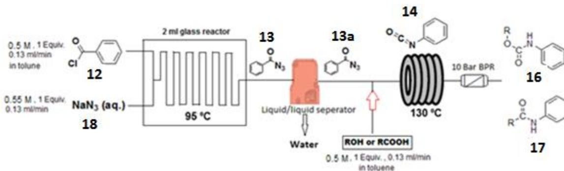
**Figure 15** General continuous flow system used in multi-step synthesis of carbamates and amides via Curtius rearrangement.
