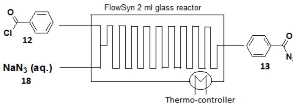
**Figure 8.** Schematic manifold for benzoyl azide synthesis optimisation in toluene.
