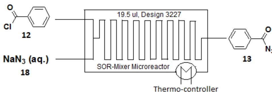
**Figure 2.** Schematic manifold used for benzoyl azide synthesis and optimisation studies.
