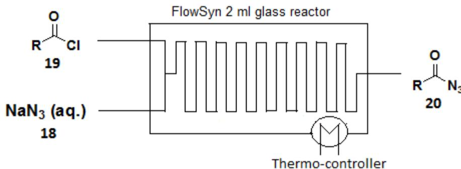
**Figure 12.** Continuous flow system for acyl azide synthesis.
