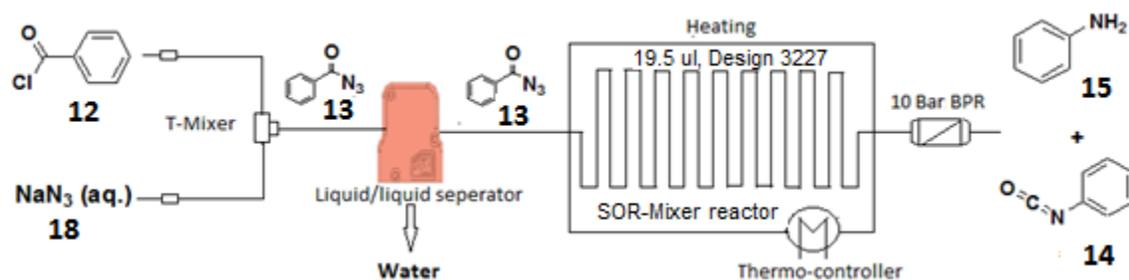
**Figure 6.** Water removal from the system attempt using a Zaiput liquid/liquid separator.
