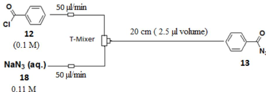
**Figure 3.** Schematic diagram of a simple continuous flow system for benzoyl azide.
