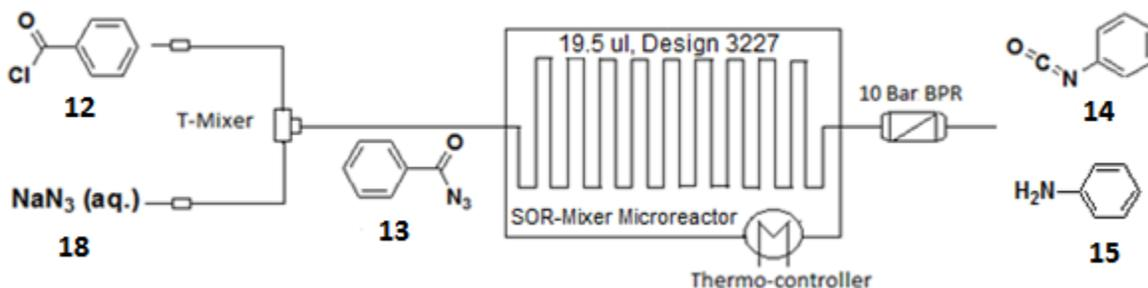
**Figure 4.** Proposed schematic diagram for multistep phenyl isocyanate synthesis in a continuous flow system.
