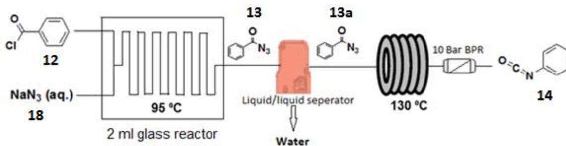
**Figure 13** Use of Liquid/liquid separator towards Curtius rearrangement reaction.
