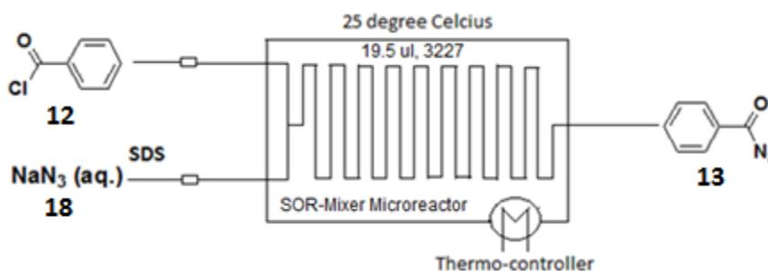
**Figure 7.** Schematic manifold used for benzoyl azide synthesis in toluene using SDS as a catalyst in Labtrix flow system.
