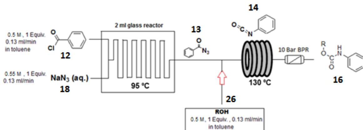
**Figure 17** Carbamate synthesis in the absence of a liquid/liquid separator.
