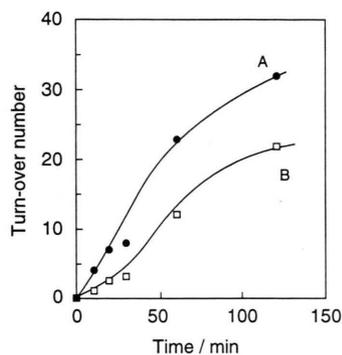
Fig. 5. Time course of turn-over numbers (= [mole of product]/[mole of iron(III) complex]) of products from tetrahydrofuran. A: tetrahydrofuran-2-hydroperoxide; B:  $\gamma$ -butyrolactone.
