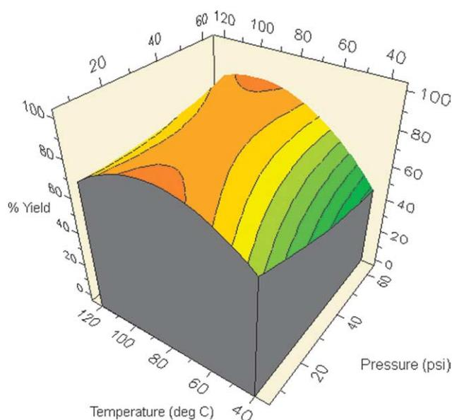
**Figure 2.** Temperature and pressure response surface for the cyclization of **3**.
