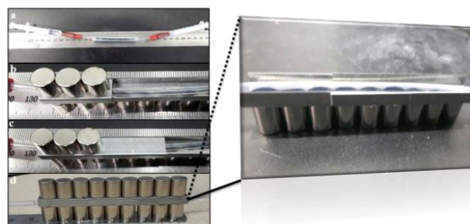
Figure 1. Reversible fixation of magnetic nanoflakes to tubes with external magnets.
