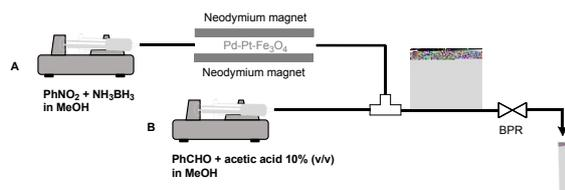
A continuous reductive amination was performed using NH<sub>3</sub>BH<sub>3</sub> through reversible magnetic bimetallic fixation under room temperature.
