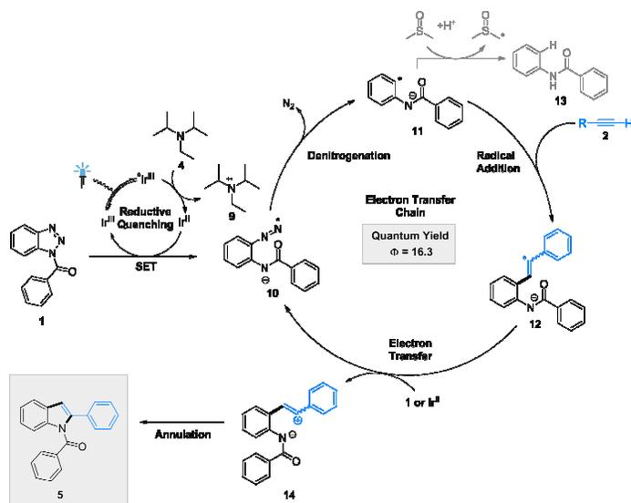
**Scheme 5. Proposed mechanism for the photoinitiated denitrogenative synthesis of 2-substituted indoles.**
