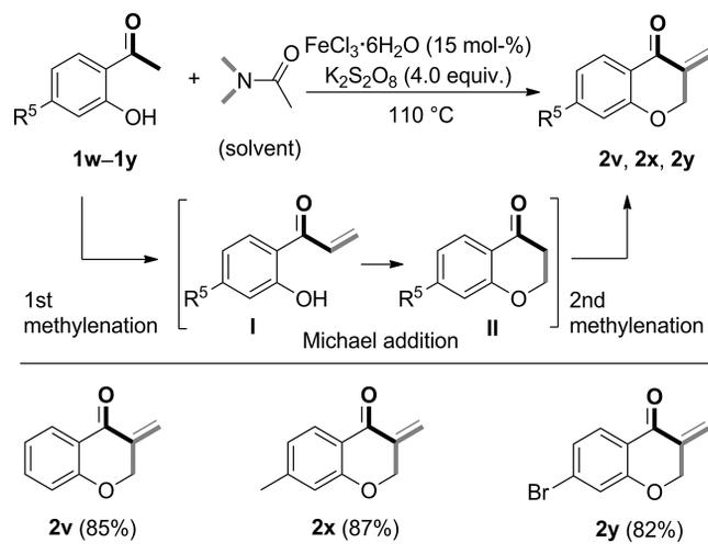
Figure 1. Two-fold  $\alpha$ -methylation of *ortho*-hydroxyacetophenones. Reaction conditions: **1** (0.5 mmol),  $\text{FeCl}_3 \cdot 6\text{H}_2\text{O}$  (0.075 mmol),  $\text{K}_2\text{S}_2\text{O}_8$  (2.0 mmol), DMA (2.0 mL),  $110^\circ\text{C}$ , 4 h, under air, isolated yields.
