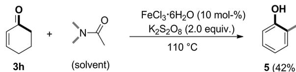
Scheme 2.  $\alpha$ -Methylation and cascade aromatization of **3h**.
