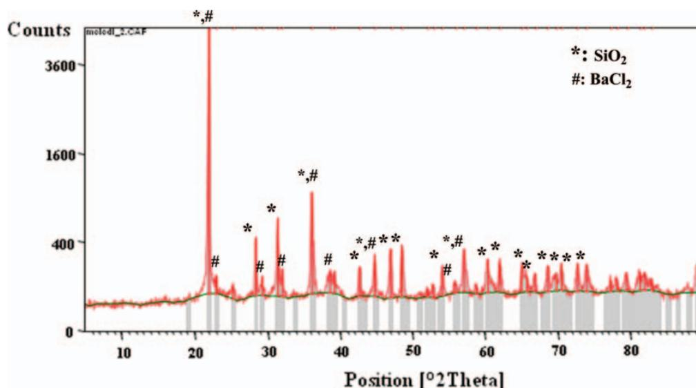
Fig. 1 XRD pattern of BaCl<sub>2</sub>-nano SiO<sub>2</sub>.
