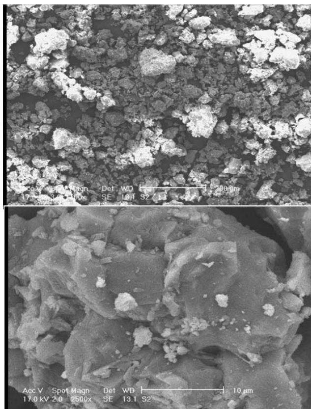
Fig. 2 SEM micrographs of barium chloride dispersed on silica gel nanoparticles (BaCl<sub>2</sub>-nano SiO<sub>2</sub>).
