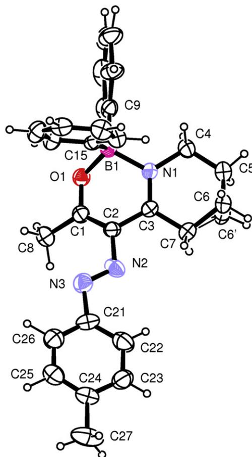
**Fig. 1.** ORTEP view of compound **5b** displaying the thermal ellipsoids at 30% probability. Both the disordered C6 and C6' atoms are shown.
