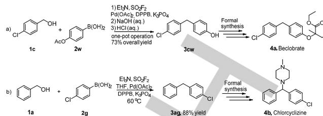
**Scheme 3.** Application of the Developed Method to Formal Synthesis of Beclobrate and Chlorcyclizine.
