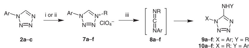
Scheme 3 Reagents and conditions: i) 1. (MeO) 2 SO 2 ; 2. ClO 4 − ; ii) t -BuOH, HClO 4 ; iii) NaN 3 (2.0 equiv), Et 3 N·HCl (2.0 equiv), MeCN, DMSO, 70 °C, 2 h.
