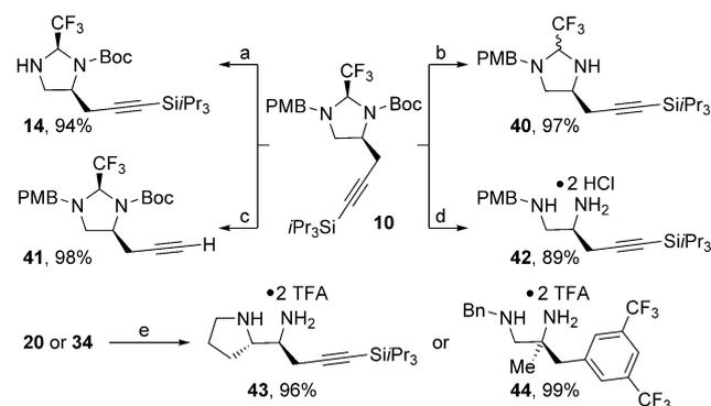
**Scheme 3.** Orthogonal deprotection. Reaction conditions: a) DDQ, MeCN,  $H_2O$ , RT; b) microwave irradiation (160 °C),  $H_2O$ /Ethanol; c) TBAF, THF, 0 °C to RT; d) HCl, MeOH, –40 °C to RT; e) TFA,  $CH_2Cl_2$ , then MeOH, 0 °C to RT.
