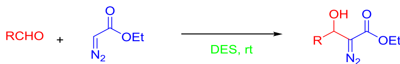
Scheme 1. The aldol-type coupling by the reaction of various aldehydes with ethyl diazoacetate (EDA)
