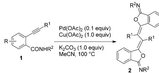
Scheme 2. Cyclizative dimerization of *o*-(1-alkynyl)benzamides leading to axially chiral bis-iminobenzoisofurans.
