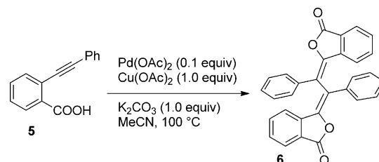
Scheme 3. Cyclizative dimerization of *o*-(1-alkynyl)benzoic acid **5**.
