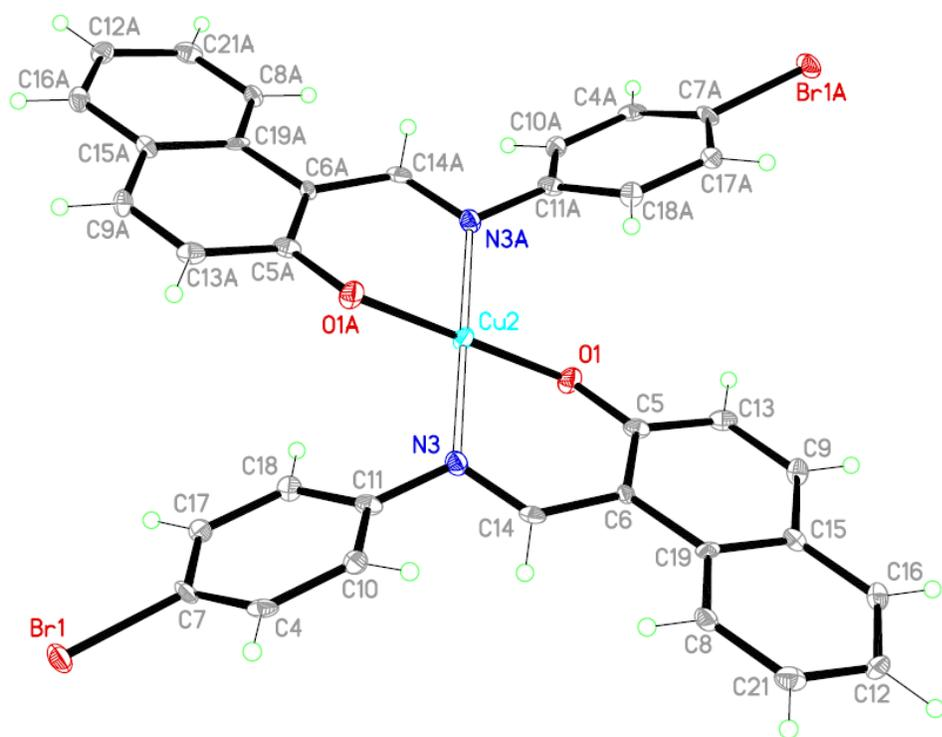
Figure 2. The ORTEP of 1 with atoms labelling and ellipsoids probability of 40%. The A suffix is for symmetry code,  $-x + 1, -y, -z + 1$ .
