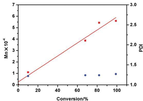
Fig. 4 Plot of  $M_n$  (■) and polydispersity (●) versus monomer conversion in the ROP of  $\epsilon$ -CL initiated by **2c** (Table 2, entries 3, 9–11).
