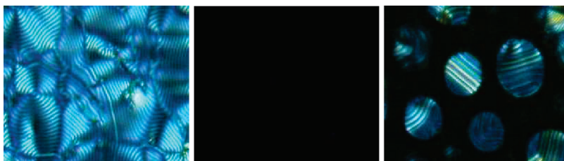
Figure 9. Crossed polarized optical texture micrograph of 10 wt % of 7a in a nematic LC host 5CB at 40 °C before UV irradiation (left), after UV irradiation at 310 nm for 30 s (middle), and followed by visible light at 670 nm for 60 s (right).
