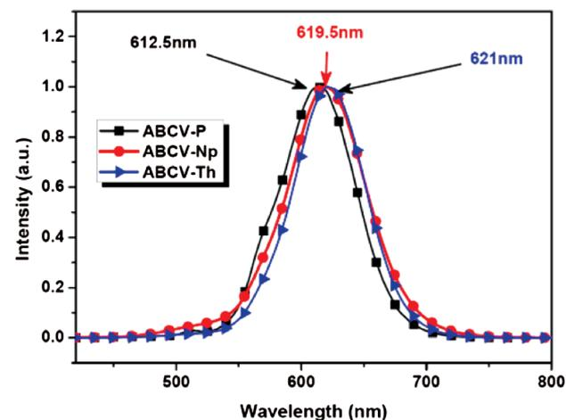
**Fig. 7.** Normalized EL spectra of ABCV-P, ABCV-Np and ABCV-Th with the device structures of ITO (100 nm)/NPB (40 nm)/red emitters (30 nm)/BCP (10 nm)/Alq<sub>3</sub> (20 nm)/Liq (2 nm)/Al (100 nm), in which red emitters are ABCV-P, ABCV-Np and ABCV-Th.
