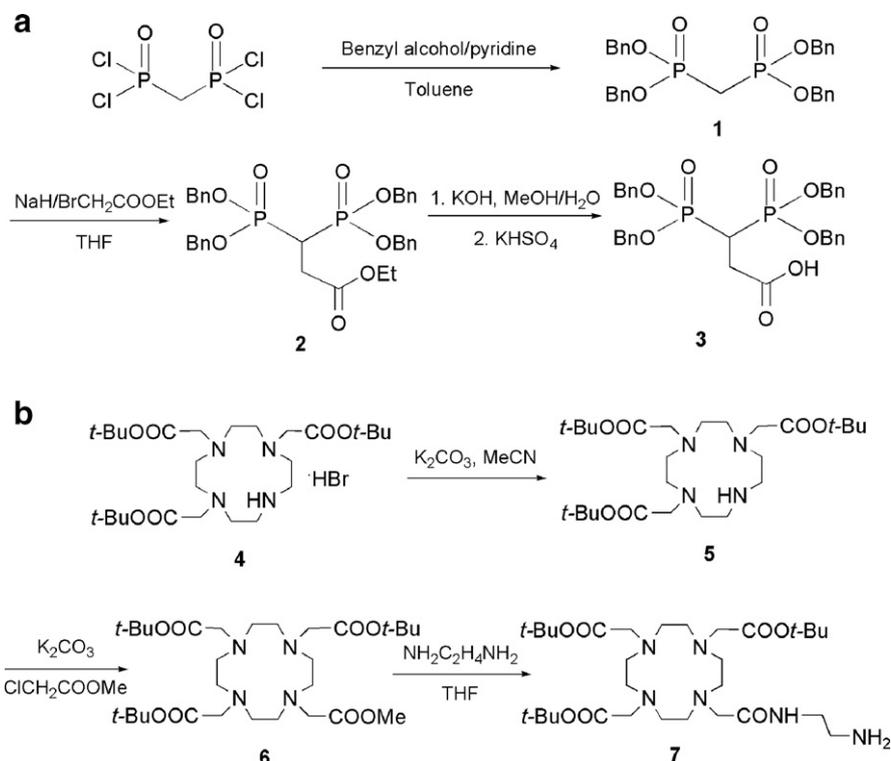
**Scheme 1.** Synthesis of derivatives of (a) a bisphosphonate and (b) DOTA.
