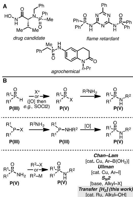
**Fig. 1:** (A) Representative examples of phosphinic amides with different applications. (B) Overview of synthetic methods for preparing phosphinic amides.
