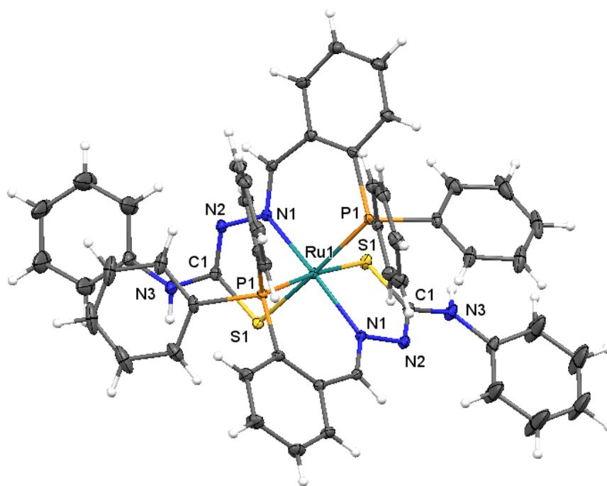
**Fig. 1.** Molecular structure of [Ru(PNS-Ph)<sub>2</sub>] (2) with thermal ellipsoids at the 50 % probability level.
