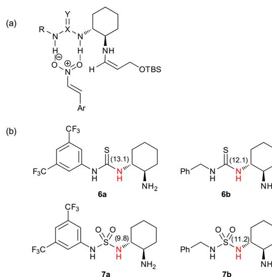
**Figure 2.** (a) Plausible transition state; (b) pK<sub>a</sub>'s of sulfamides versus thioureas.
