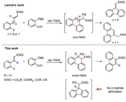
Inspired by Larock's work, we envisioned that 9,10-phenanthrenes would be produced via arylpalladium(II) aryne insertion and intramolecular *endo*-Heck reaction when the R group is not a proton (Scheme 1). Herein, we report our results on the synthesis of 9,10-phenanthrenes via palladium-catalyzed annulation of in situ generated arynes and readily available *o*-halostyrenes and its application in the formal total synthesis of the anticancer natural alkaloid ( $\pm$ )-tylophorine.
