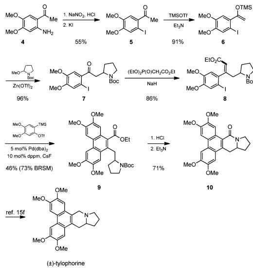
a 46% yield of phenanthrene **9** (73% based on recovery of starting material **8**). Deprotection of the Boc group followed by intramolecular cyclization generated lactam **10**, which can be reduced to ( $\pm$ )-tylophorine in one step via a literature procedure.<sup>15f</sup>
