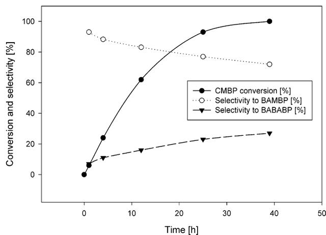
**Figure 3. CMBP hydrogenation with in situ BOC protection. Reaction conditions: T = 298 K, H<sub>2</sub> 500 psi, IPA 30 mL, H<sub>2</sub>O 20 mL, BOC 4 equiv of CMBP, CMBP 0.5 mmol, Raney Cobalt (doped with Ni, Cr) 0.03 g.**
