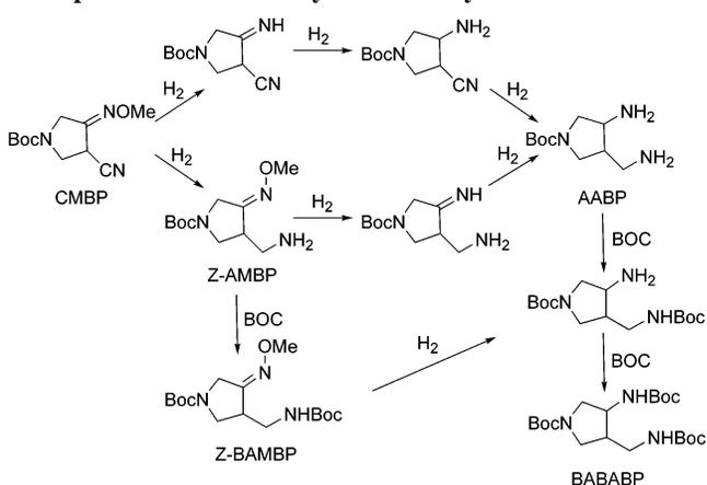
protection is proposed on the basis of these observations in Scheme 4. In this scheme, the reaction pathway from CMBP to Z-BAMBP via Z-AMBP is dominant, and hydrogenation of Z-BAMBP to BABABP is negligible.
