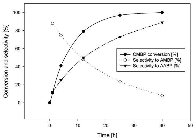
**Figure 2. CMBP hydrogenation without in situ BOC protection. Reaction conditions: T = 313 K, H<sub>2</sub> 500 psi, IPA 30 mL, H<sub>2</sub>O 20 mL, CMBP 0.5 mmol, Raney Cobalt (doped with Ni, Cr) 0.03 g.**
