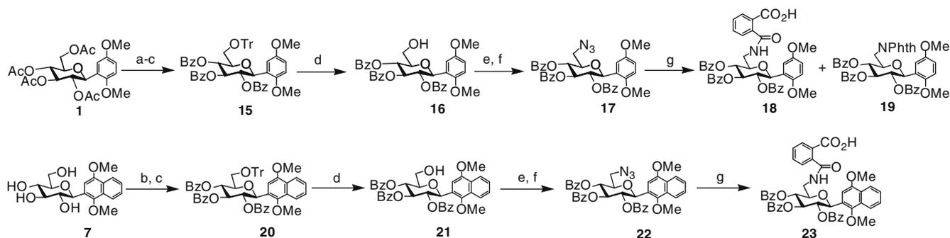
**Scheme 2.** Reagents and conditions: (a) MeONa, MeOH; (b) TrCl, pyr.; (c) BzCl, 61% (d) TFA, CH<sub>2</sub>Cl<sub>2</sub>, H<sub>2</sub>O, **16**: 79%, **21**: 83%; (e) MsCl, TEA; (f) NaN<sub>3</sub>, DMF, 57%; (g) phthalic anhydride, Me<sub>3</sub>P, CH<sub>2</sub>Cl<sub>2</sub> for **18** and **19** (**18**: 47%, **19**: 22%), THF for **23** (90%).
