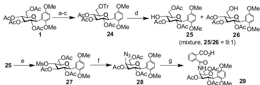
**Scheme 3.** Reagents and conditions: (a) MeONa, MeOH; (b) TrCl, pyr.; (c) Ac<sub>2</sub>O, 89% (d) TFA, CH<sub>2</sub>Cl<sub>2</sub>, H<sub>2</sub>O, 78%; (e) MsCl, TEA, 55%; (f) NaN<sub>3</sub>, DMF, 71%; (g) phthalic anhydride, Me<sub>3</sub>P, CH<sub>2</sub>Cl<sub>2</sub>, 74%.
