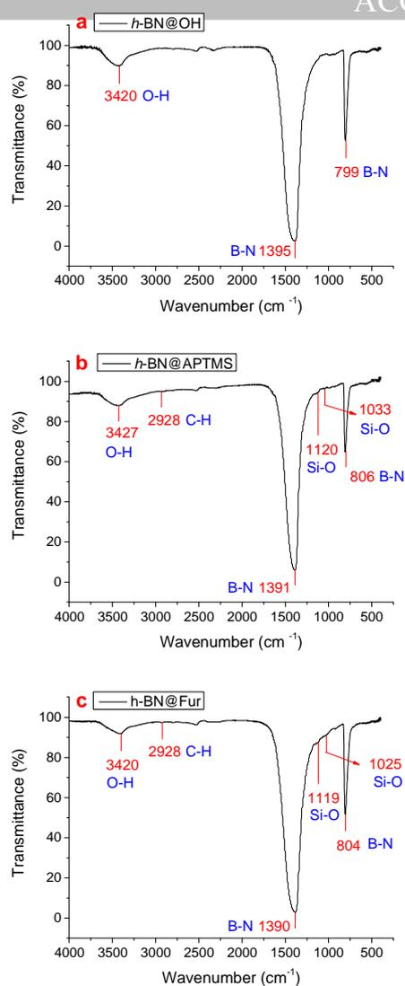
**Figure 2.** FT-IR spectra of (a) *h*-BN@OH, (b) *h*-BN@APTMS, (c) *h*-BN@Fur.
