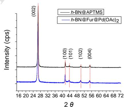
**Figure 4.** XRD patterns of *h*-BN@APTMS and *h*-BN@Fur@Pd(OAc)<sub>2</sub>.
