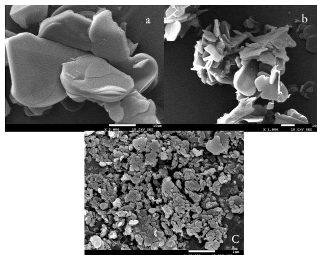
**Figure 1.** SEM of (a) pristine  $h\text{-BN}$ , (b)  $h\text{-BN@OH}$  and (c)  $h\text{-BN@Fur@Pd(OAc)}_2$ .
