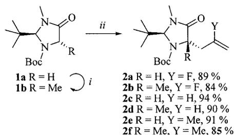
Scheme 1. Stereoselective alkylations of (*S*)-Boc-BMI reagents and conditions: i. LDA, DMPU, THF, MeI,  $-50^{\circ}\text{C}$ , 3 h, 96%; ii. LDA, DMPU, THF,  $\text{CH}_2=\text{CYCH}_2\text{X}$ ,  $-50^{\circ}\text{C}$ , 3 h
