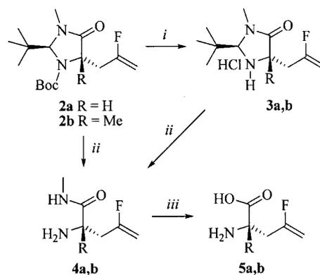
Scheme 2. Deprotection reactions of the alkylation products – reagents and conditions: i. HCl/MeOH, room temp., 1 h; ii. 1 N HCl, MeOH/ $\text{H}_2\text{O}$ , reflux, 3 h; iii. (a) 2 N KOH/ $\text{H}_2\text{O}$ , reflux, 2 h; (b) propylene oxide, EtOH, reflux, 30 min
