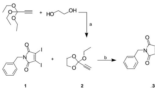
**Scheme 1.** Synthesis of enediyne **3**. a) succinic acid,  $120 \text{ }^\circ\text{C}$ , 2h; b) CuI, NHC-PdCl<sub>2</sub>-3-chloropyridine, DIPEA, THF/ toluene,  $20 \text{ }^\circ\text{C}$ , 15 h.
