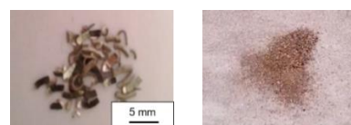
Figure 1. Photographs of Ti–Pd turnings (left) and Ti–Pd(Hy) powder (right).
