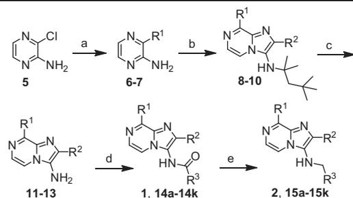
**Scheme 2.** Preparations of substrates for the cyclization study. Reaction conditions: (a) morpholine or BnNH<sub>2</sub>, NMP, DIPEA, 120–130 °C, 12 h; (b) Yb(OTf)<sub>3</sub>, 2-isocyanato-2,4,4-trimethylpentane, R<sup>2</sup>CHO, MeOH, 65 °C, 2 h; (c) HCl/EtOAc, MeOH, 25 °C, 8 h; (d) R<sup>3</sup>COOH, HOBT, EDCI, TEA, DCM, RT, 8 h; (e) BH<sub>3</sub>–THF complex, THF, 80 °C, 1 h. See Table 1 and supporting information for structural and experimental details.
