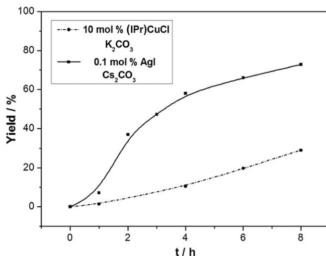
**Fig. 1.** Plot of yield versus time for the carboxylative coupling reaction catalyzed by (IPr)CuCl and AgI. Yields were determined by LC.
