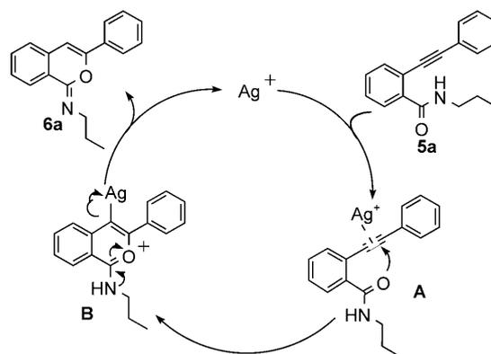
**Scheme 2.** Possible mechanism for the Ag(I)-catalyzed intramolecular cyclization.
